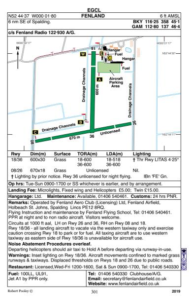
Reproduced with the kind permission of Pooleys Flight Equipment Limited.
