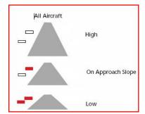
slope guidance by use of **red** and white light signals, which are interpreted below. The system is installed on the left side of Runway 18 as seen from the approach, providing an indication to the Pilot of a suitable glide slope to land adjacent to the VASI but maintaining safe clearance on approach crossing the road. (Note: At Fenland, these may be known by their old term of 'LITAS').
