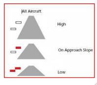
slope guidance by use of **red** and white light signals, which are interpreted below. The system is installed on the left side of Runway 18 as seen from the approach, providing an indication to the Pilot of a suitable glide slope to land adjacent to the VASI but maintaining safe clearance on approach crossing the road. (Note: At Fenland, these may be known by their old term of 'LITAS').
